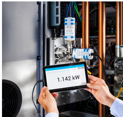
An android tablet becomes an RF power meter
