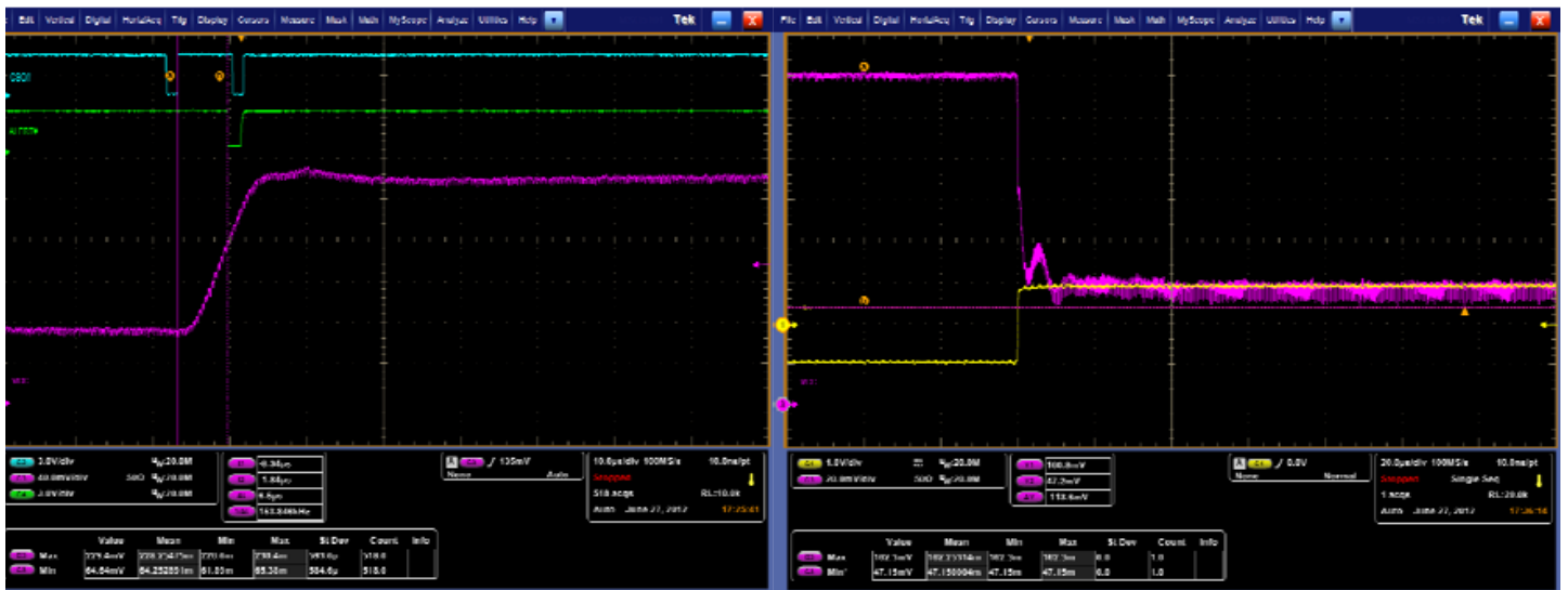
Figure 12. Response to a 1.05-V to 1.2-V setpoint transient at 108-A load (left) and a 34-A to 165-A load transient (right).
